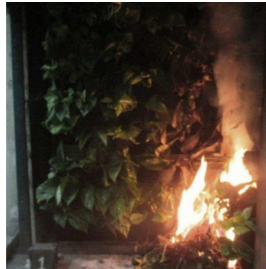
LW test specimen during and post SBI test
