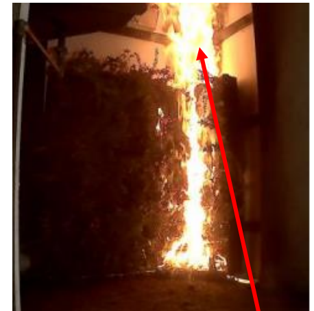
Flame from cavity between LW and support wall Węgrzyńska et al 2023
