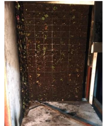
SBI test with plants trimmed back to the compost
